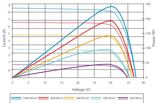
Excellent performance under weak light conditions: at an irradiation intensity of 200 W/m<sup>2</sup> (AM 1.5, 25 °C), 95.5% or higher of the STC efficiency (1000 W/m<sup>2</sup>) is achieved
