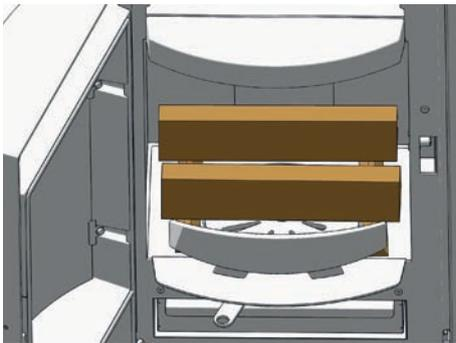
2. Now place further pieces of chipboard in crossways layers on top of the logs and place a firelighter on the left underneath the chipboard (some uncoated paper can be placed underneath the chipboard instead of using a firelighter).
