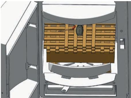
3. Open the riddle grate completely and now light the firelighter (or the uncoated paper) and close the combustion chamber door. “Correct heating up” primarily counteracts excessive smoke during heating up.
