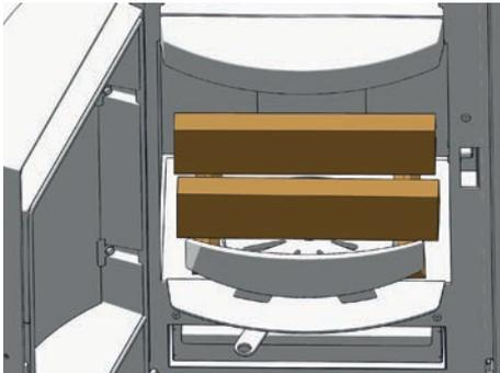
Now place further pieces of chipboard in crossways layers on top of the logs and ideally you should place a firelighter on top of the chipboard (some uncoated paper can be placed underneath the chipboard instead of using a firelighter).
