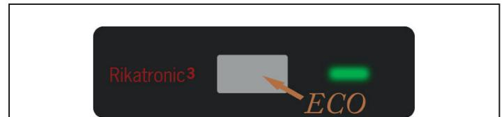
If the room to be heated and the stove are already at temperature, continued operation with lower heat output and log addition is possible.
