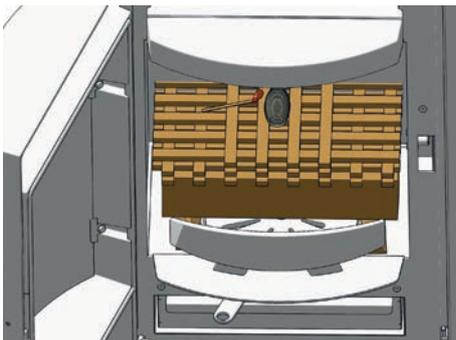
Now light the firelighter (or the uncoated paper) and close the combustion chamber door. "Correct heating up" primarily counteracts excessive smoke during heating up.
