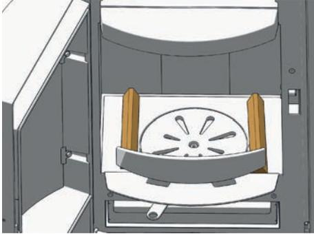
Place 2 – 3 smaller (highly flammable) logs crossways on top of this chipboard.
