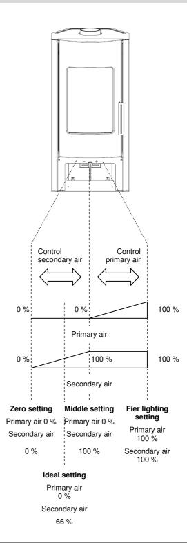
There is a lever on the rear of the wood handle that serves as a stop to prevent complete closure of the slide control. The air regulator can be closed by pressing the lever forwards. Complete closure is only permitted when cold; it is strictly prohibited during operation (deflagration hazard).
